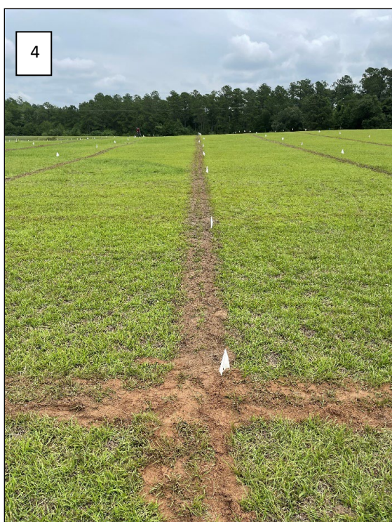
Figure 3-4 Installation of ERT Electrode Cables
