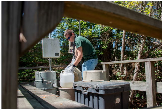
A Teledyne ISCO Sampler Jug is Removed Before Being Taken to the Lab for Analysis.
