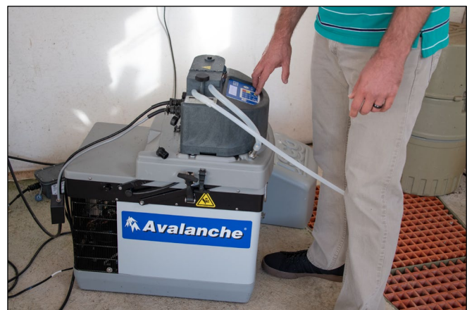
A Refrigerated Sampler Allows for Remote Temperature Verification.
