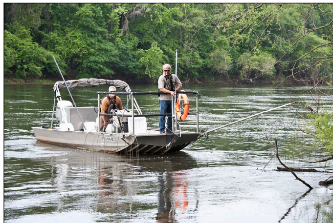
SRS Samples Fish from the Savannah River Using Electrofishing Methods. Radionuclide Concentrations in Fish Harvested from the Steel Creek Mouth are Used in the Representative Person Dose Calculations.
