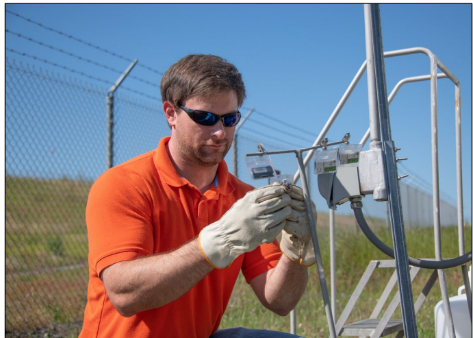
SRS Employee Measures Environmental Gamma Exposure Rates with OSLDs Placed Across the Site.
