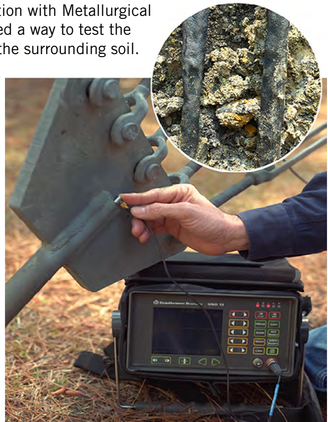
SoundAnchor™ device testing integrity of anchor rods (inset: Corroded anchor rod at test location)
